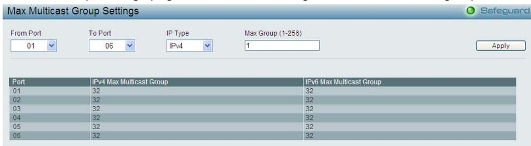
Figure 5.59- Configuration > IGMP Snooping > Max Multicast Group Settings
