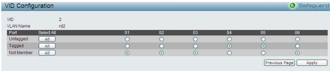
Figure 5.45 - Configuration > 802.1Q VLAN > VID Assignments
