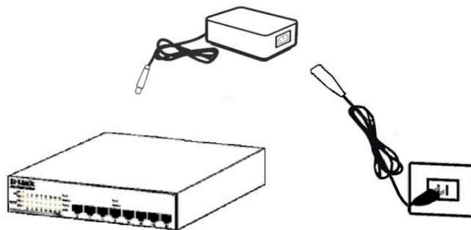
Figure 2.3 – Plugging the switch into an outlet
