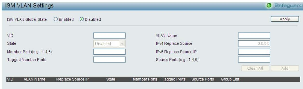
Figure 5.54 - Configuration > IGMP Snooping > ISM VLAN Settings
